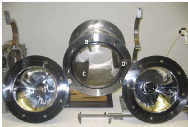
Figure 24: Photograph showing the high-gloss polished inside of the dustiness drum. Also note the three lifter vanes marked a, b, and c at each 120° in the drum.
