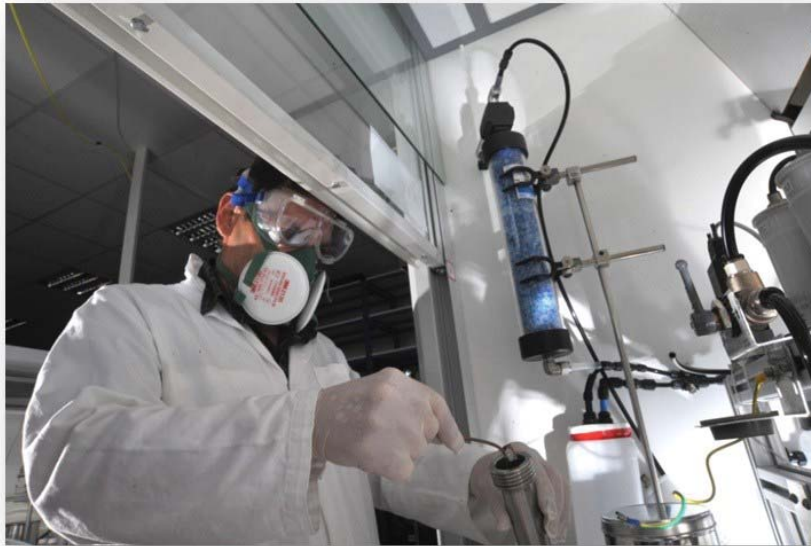
Figure 33: Operator introducing a NM sample into the Vortex Shaker positioned in the variable volume fume hood used at INRS.
