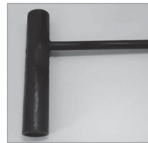
Figure 18: Ejector with side sampling junction
