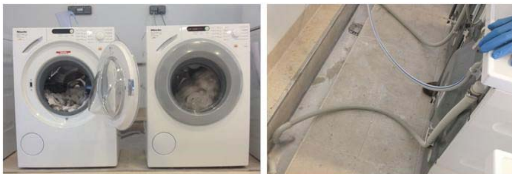
Figure 2: Conventional washing machines (left) used for the lab-washing experiments in procedure 2 and disposition of the evacuation tube to collect the laundering waters (right).
