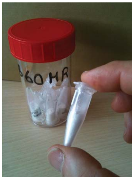
Figure 29: Microcentrifuge tube filled with a NM sample of 0.5 \text{ cm}^3 for a dustiness test according to the VS method.
