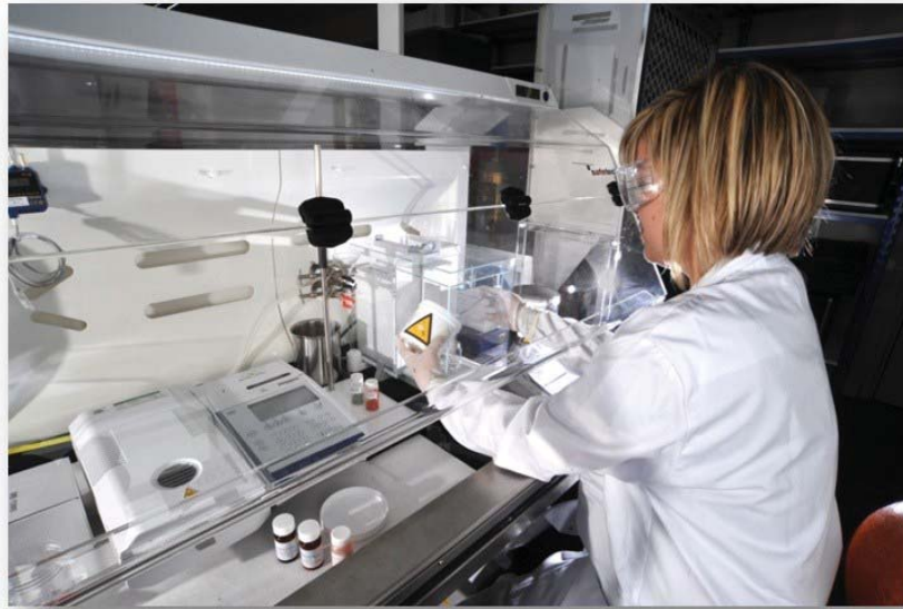
Figure 32 : Operator during NM sample preparation (weighing and water content measurement) in the powder handling enclosure at INRS.
