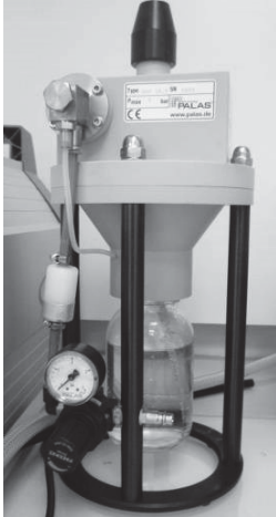
Figure 14: PALAS AGF 10 nebuliser and NaCl solution
