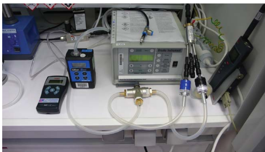
Figure 31 : View of the set-up designed to collect emitted particles on grids for EM observations.
