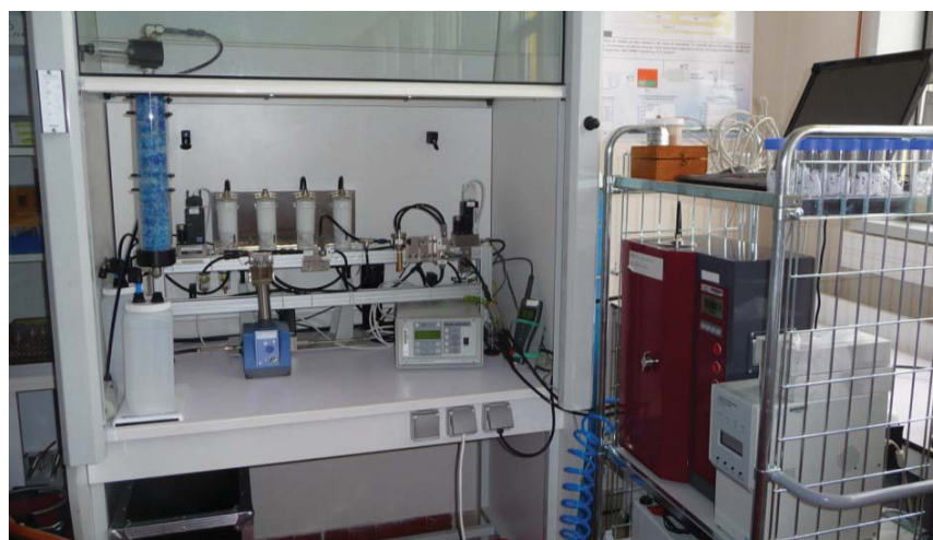
Figure 30 : Overview of the vortex shaker set-up positioned in the variable flow fume hood at INRS.
