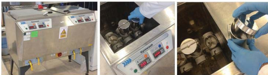
Figure 1: GyroWash machine used to perform the lab-washing experiments in procedure 1.
