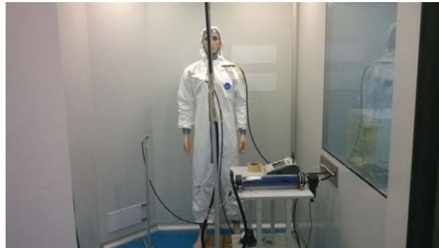
Figure 6: Tests of penetration of airborne nanoparticles in suits with a mannequin
