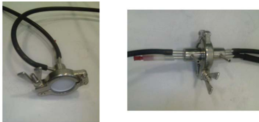
Figure 4: Set up for gloves testing the penetration of airborne nanoparticles.
