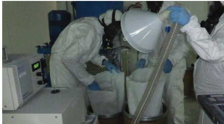
Figure 8: Portable captor hood placed during the transfer of NM.
