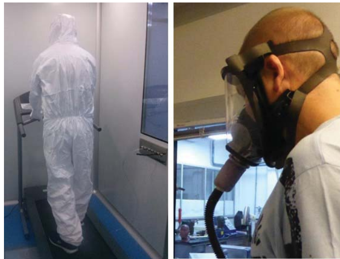
Figure 2: Test Subject for RPE with NaCl on a treadmill.
