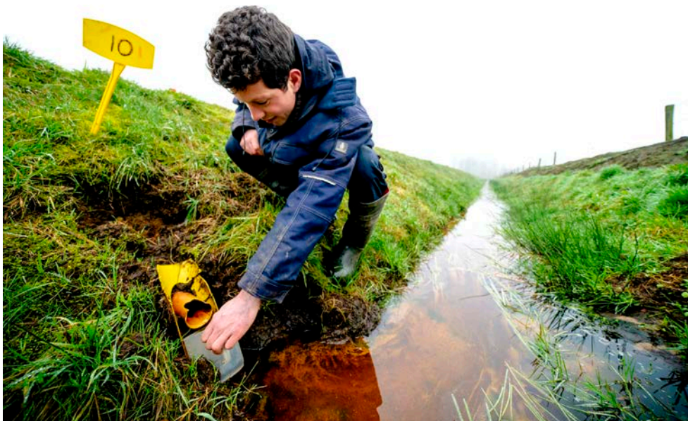
Figure 3.6 Sampling of drain water.
