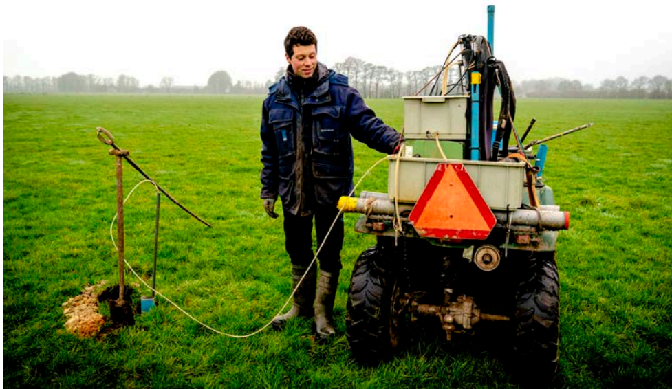
Figure 3.5 Sampling of groundwater in the Sand region using a temporary borehole.
