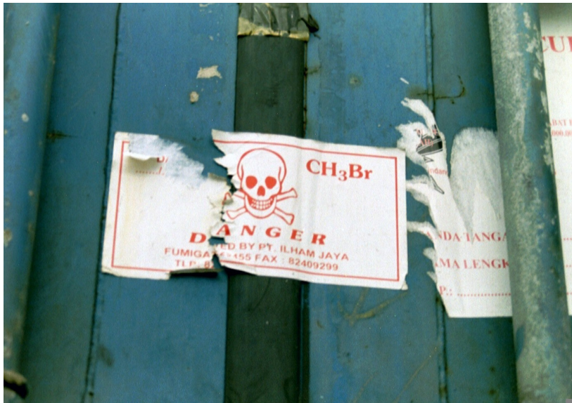
Figure 1 Warning sticker on a fumigated container.
